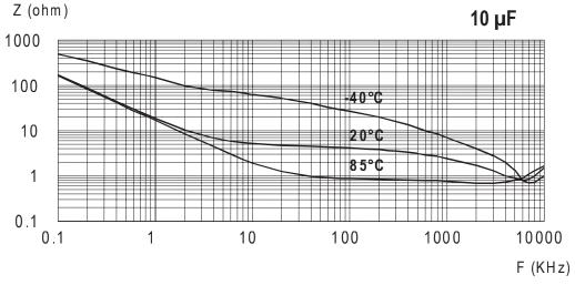
R<sub>e</sub> is the most temperature-dependent component of an electrolytic capacitor equivalent circuit. Electrolyte resistivity will decrease if temperature rises.
